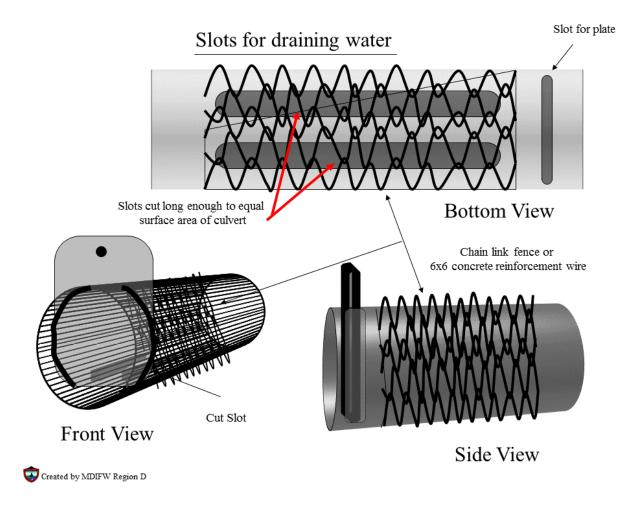
NOTE: This same design can be used for smaller diameter culverts used as water levelers. Heavy-duty livestock dishes can also be used to block the upstream end of the leveler and are easier to install.
