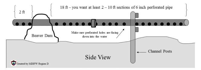
Note: A single culvert can be used in place of multiple drainage pipe.
