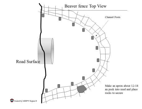
Standard fence with drainage pipes as water levelers
